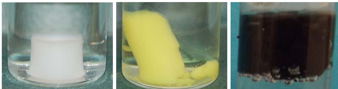
Figure 4.7. Pictures of a (left) ZnS wet gel; (middle) \text{Cd}^{2+} and (right) \text{Pb}^{2+} exchanged wet gel, showing the specific color change and the conservation of the 3D gel monolith integrity upon the cation exchange. (The size of the monoliths is not to scale, nor does it represent a series in which a particular ZnS monolith was exchanged)
